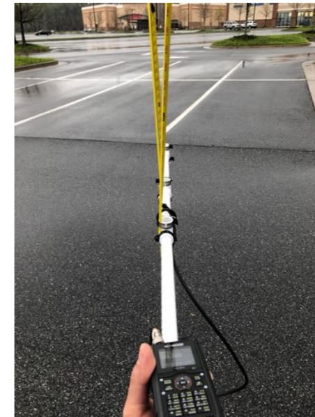
Sniffer – the radio receiver used to find the fox
